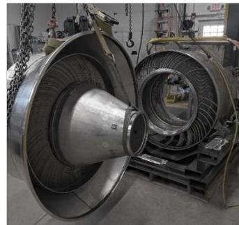
This is a photo of our turbine and heat exchanger – one of several breakthrough components that make 247Solar Plants an ideal solution for producing round-the-clock clean power without batteries or backup gensets.
